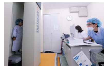
Measuring radioactivity inside the human body using the whole body counter (Fukushima Red Cross Hospital) ©Nobuyuki Kobayashi
